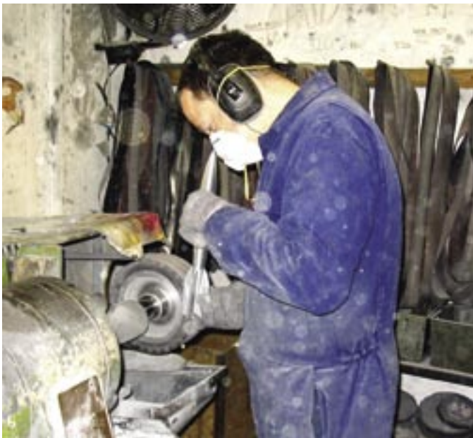
6. Dressing the casting on a finishing wheel, to remove split lines and feeder witnesses.
