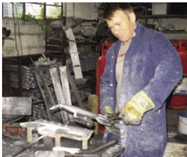
3. Removing the casting from the die, with the feeder sprue and overflow block attached.
