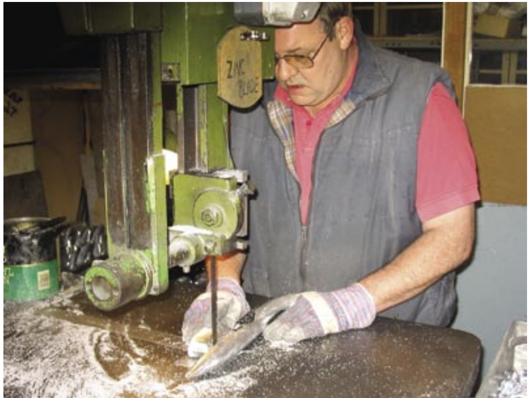
5. Removing sprue and overflow block with a band-saw.
